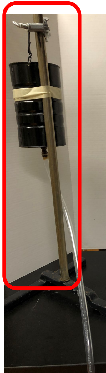
Experiment mimicking IV bag and needle in arm
